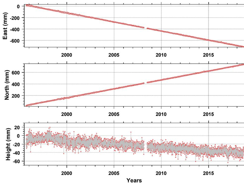
**Figure 4-2:** An example of a position time series for the cGNSS site at Otago University (OUSD). *Source:* P Denys (Univ. of Otago).
