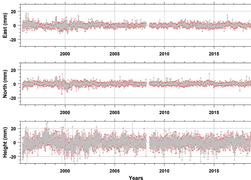
**Figure 4-3: Detrended position time series using the same data as in Figure 4-2.** Source: P Denys (Univ. of Otago).
